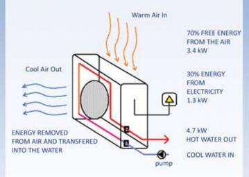
As the ambient temperature changes, the heating output of a heat pump will vary. However, even when temperatures are cooler, the heat pump continues to transfer heat between air and water. SIRAC heat pumps are designed to operate between -15°c and 40°c ambient temperature. On a typical South African summer day, the heat pump will provide 4kW of heating with only 1kW of electrical input. By contrast electrical elements require 4kW of electrical energy to generate 4kW of heat energy.
