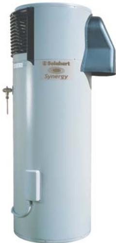
**Electric Boost:** The storage cylinder comes fitted as standard with a 3.6 kW element, however elements ratings from 1.8kw through to 6.0kw are available. The system is available in 3 tank sizes; 270 litres, 340 litres & 430 litres.
